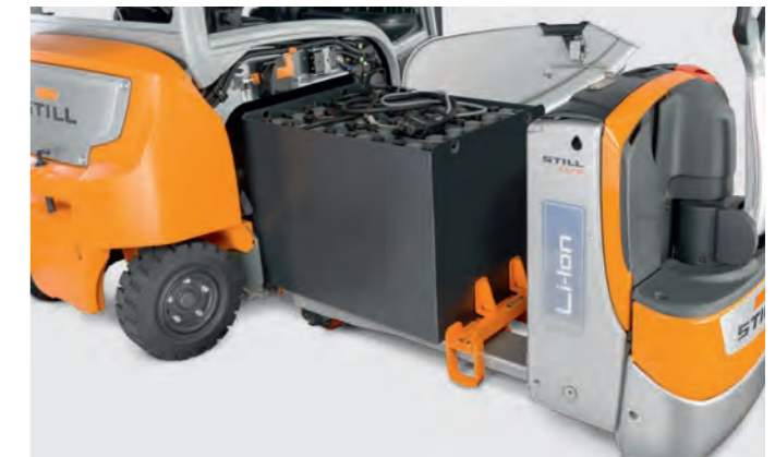
Battery change with electric pallet truck
