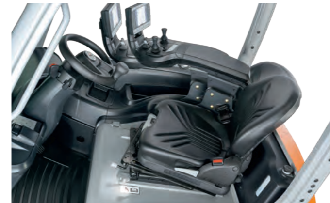
Swivel seat for comfortable reversing
