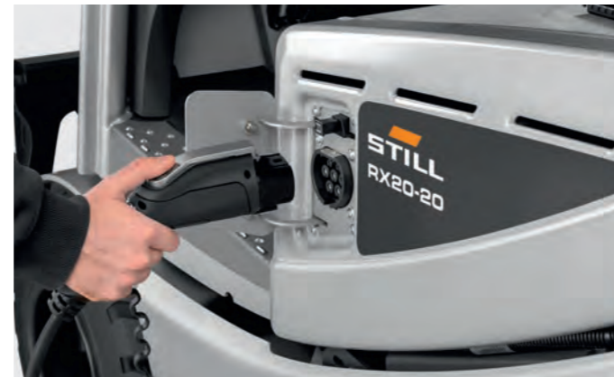
Optional onboard charger for decentralized charging without battery change
